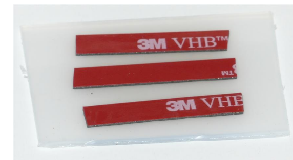
Tape to secure wires.
